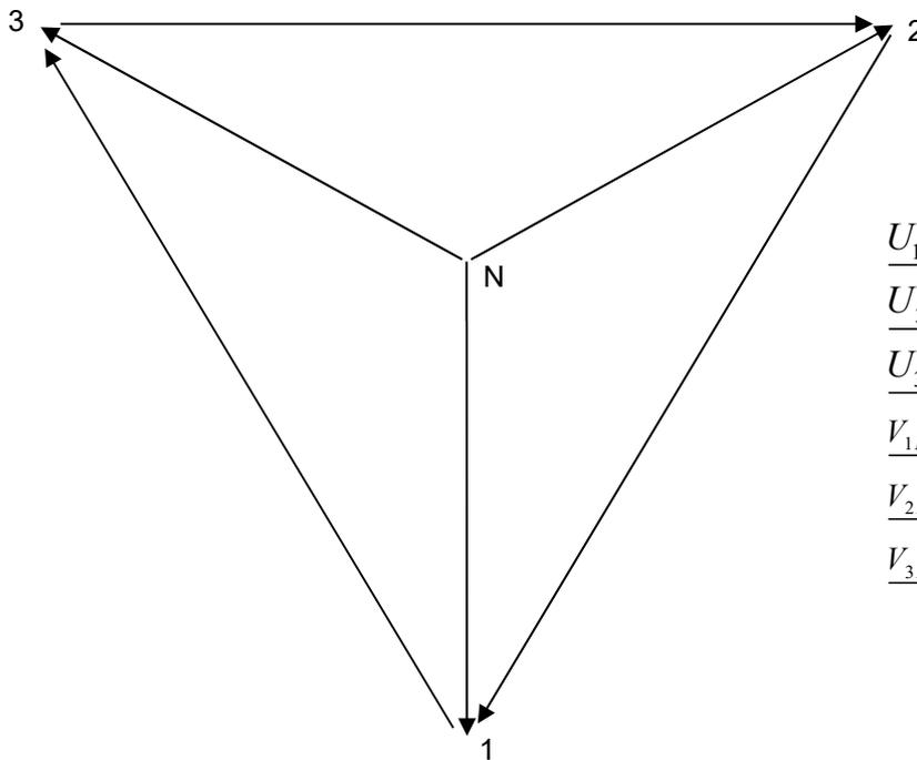
$$\begin{aligned} \underline{U}_{12} &= U \angle 240^\circ \\ \underline{U}_{23} &= U \angle 0^\circ \\ \underline{U}_{31} &= U \angle 120^\circ \\ \underline{V}_{1N} &= (U/\sqrt{3}) \angle -90^\circ \\ \underline{V}_{2N} &= (U/\sqrt{3}) \angle 30^\circ \\ \underline{V}_{3N} &= (U/\sqrt{3}) \angle 150^\circ \end{aligned}$$
