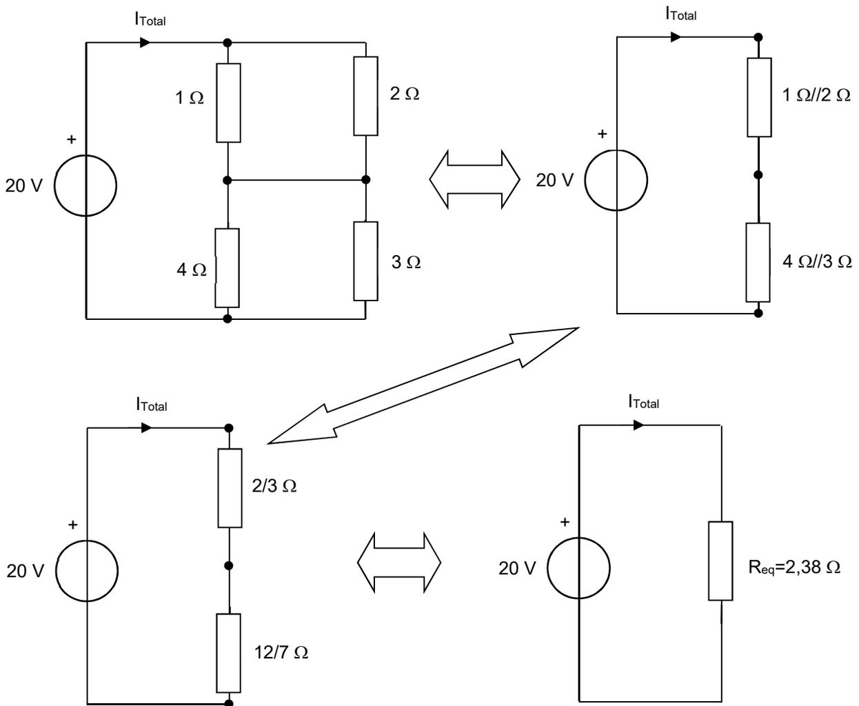
$$R_{eq} = \frac{2}{3} + \frac{12}{7} = \frac{50}{21} \approx 2,38 \Omega \Rightarrow I_{Total} = \frac{20}{\frac{50}{21}} = \frac{42}{5} \approx 8,4 \text{ A}$$
