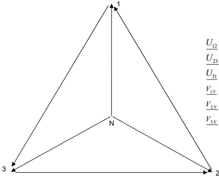
$$\begin{aligned} \underline{U}_{12} &= U \angle 120^\circ \\ \underline{U}_{23} &= U \angle 0^\circ \\ \underline{U}_{31} &= U \angle 240^\circ \\ \underline{V}_{1N} &= (U/\sqrt{3}) \angle 90^\circ \\ \underline{V}_{2N} &= (U/\sqrt{3}) \angle -30^\circ \\ \underline{V}_{3N} &= (U/\sqrt{3}) \angle -150^\circ \end{aligned}$$
