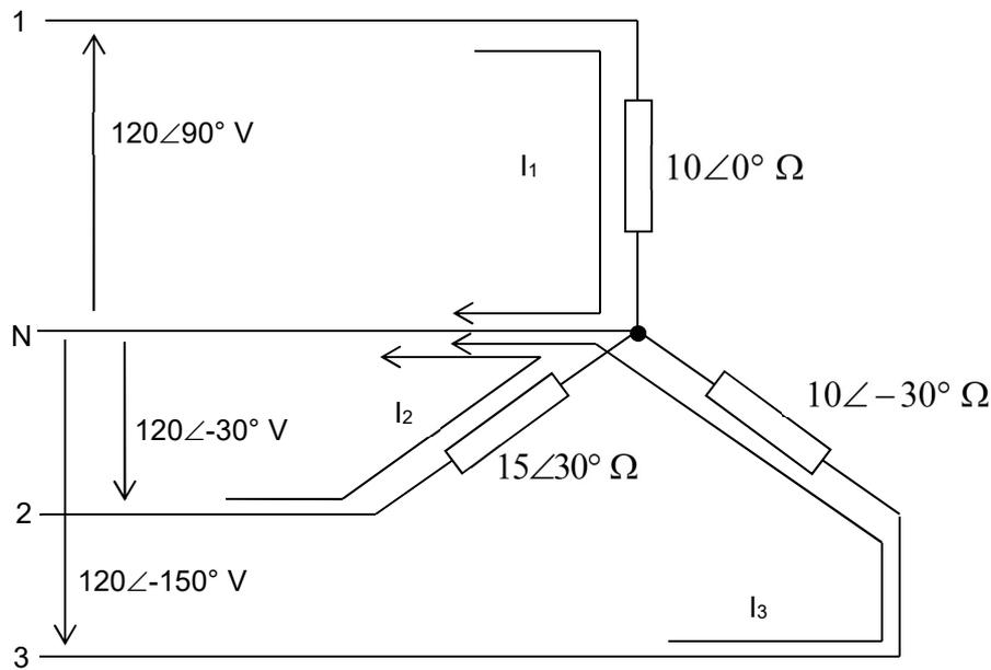
$$\underline{I}_1 = \frac{V_1}{Z_1} = \frac{120\angle 90^\circ}{10\angle 0^\circ} = 12\angle 90^\circ \text{ A}$$
