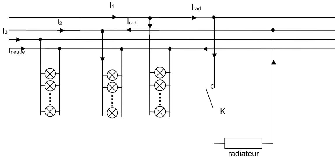
$$\underline{I_1} = \underline{I_{1Lampes}} + \underline{I_{radiateur}}$$
