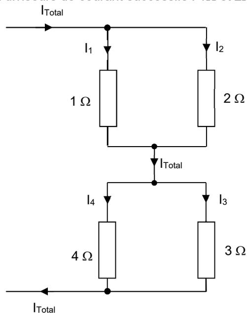
Dans  $1\Omega$  : on a  $I_1 = \frac{42}{5} \times \frac{2}{1+2} = \frac{84}{15}$  A
