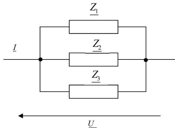
On a :  $\underline{U} = \underline{U}_1 = \underline{U}_2 = \underline{U}_3$
